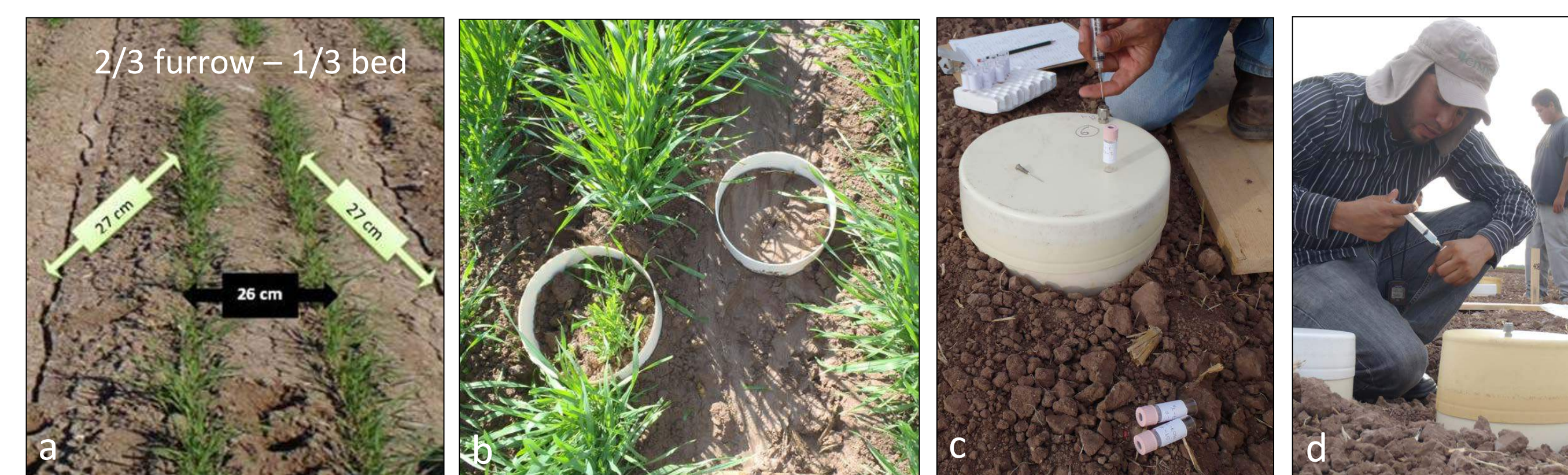
Fig. 4. Manual chamber sampling and analysis for N 2 O: a) Bed and furrow dimensions, b) chamber placement within each plot, c) gas sample extraction from chamber headspace, d) sample vial filling, e) automated gas chromatography analysis, and f) N 2 O concentration vs. sampling time ( \delta C/\delta T ) graph for N 2 O flux calculations.
